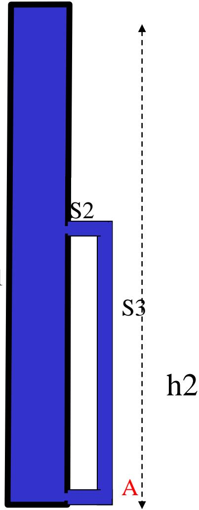
Hydrostatic pressure in **A** is proportional to  $h_2$  and varies only with  $h_2$  and is not changed by compliance in **A**, so no reservoir effect in **A**.
